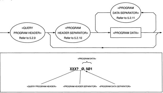
When a program header <COMMAND MESSAGE UNIT> or <QUERY MESSAGE UNIT> is followed by program data, a space is inserted between them. A program header indicates the application, function, and operation of the program. If a program header is not followed by program data, the program header solely indicates the application, function, and operation to be performed in the device.
