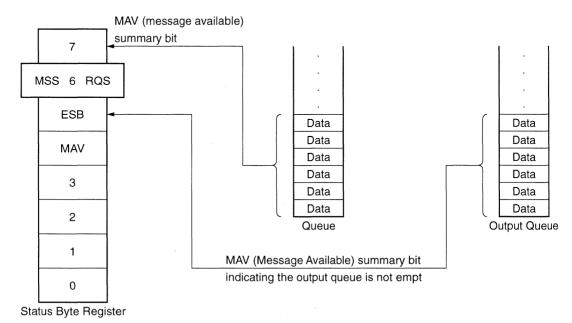
The queue that outputs an MAV summary bit to status byte register bit 4 is called an "output queue." This queue is mandatory. The queue that can output an MAC summary message to one of status byte register bits 0 to 3 and 7 is simply called a "queue." It is optional. A summary message from the register model can also be output to status byte register bits 0 to 3 and 7, so the summary message type depends on the device type.
