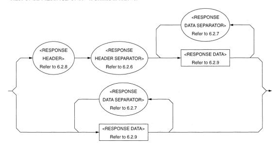
One is a response message unit with header, which returns the result of processing the program-message-set information accurately. The other is a response message unit without header, which returns only the measurement result.
